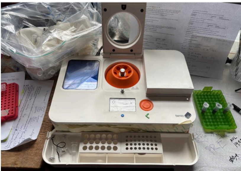
The portable benchtop Bento Lab with centrifuge and programmable PCR.
