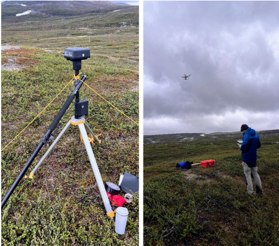
Flight operations with the DJI Phantom4RTK (20-MP RGB camera) and base station. Photo © Yajie Zhu.
